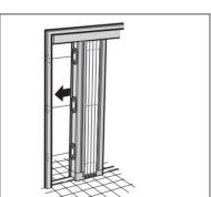
⑤ Slide the Screen Door Unit towards the door installation frame keeping the bottom of in contact with the Bottom Rail. Press firmly to attach in place.
