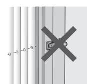
A6-A7 The screen door works by retracting the Scorpion Tail inside the Slide Bar and the Stile Post. Do not drill holes to the (aluminum) profiles and/or screw on handles or locks. If you have attempted to do this and the screen door does not work even when the screws are removed, or if the profiles are dented, you will need to replace the entire Screen Door Unit. Please consult your dealer for details.
