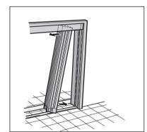
5.Re-attach the Screen Door Unit ①Close the Screen Door Unit.
