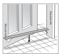
Carefully peel back the non-adhesive side of the double-sided tape on the Bottom Rail.
