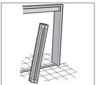
② Tilt the Screen Door Unit and remove from the Top Rail.
