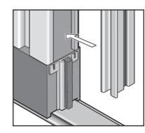
4.Re-attach the Magnet Holder Re-attach the Magnet Holder to the Slide Bar when the adjustment is complete.
