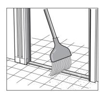
1.Clean the Bottom Rail and its surroundings Clean the Bottom Rail and its surroundings thoroughly to remove all dirt and foreign objects.
