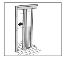
(4) Check the Screen Door Unit does not come off of rail and press firmly towards the door installation frame making sure the Anchor Plates fasten in place with an audible "click".
