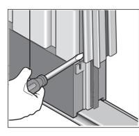
①Remove the Magnet Holder from the Slide Bar to adjust the Slide Bar inclination by adjusting the "adjust screw" inside the Slide Bar.
