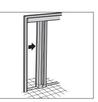
2. Remove the Screen Door Unit The Screen Door Unit can be removed easily and rinsed when it is dirty. Use a soft brush or the like to clean the pleated net and the Scorpion Tail.
