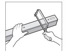
Even though the product is made to measure, if the install location is still narrower than the product, cut the Top Rail and Bottom Rail to match installation width. 3. Cut the Top Rail
