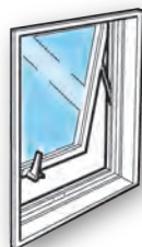
横滑り出し窓 Top-hinged outswinging window
