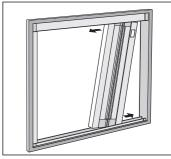
1)Confirm that "INSIDE" sticker faces inwards the room. Then tilt the insect screen and insert it diagonally.
