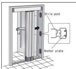
⑨ Keeping the bottom of the screen door unit in contact with the bottom rail, align the stile post with the projections of the anchor plate and press it firmly to fit the screen door unit in place.
