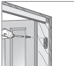
④ Provisionally place the anchor plates at the above mentioned marks after taking away the white tape from the anchor plate.
