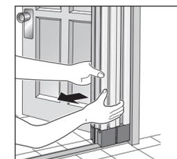
10. Screw the anchor plates to the door installation frame.
