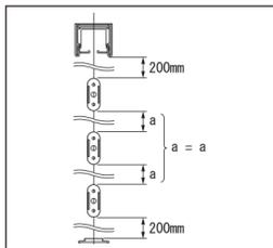
③ On the vertical center line drawn in 9-B-① check the marks at the position 200mm away from the top rail and also from the bottom rail. And also check the marks at the same distance between each anchor plate afterwards.
