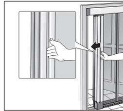
Make sure to hold the central part of the sliding bar to open & close the unit. Push it onto the door post. It easily closes as the magnet is slotted in the door post.
